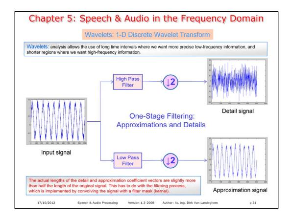
For many signals, the low-frequency content is the most important part. It is what gives the signal its identity. The high-frequency content, on the other hand, imparts flavor or nuance. Consider the human voice. If you remove the high-frequency components, the voice sounds different, but you can still tell what's being said. However, if you remove enough of the low-frequency components, you hear gibberish.
